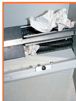
AUTOMATIC MECHANICAL FEEDING SYSTEM WITH REVOLVING FLAPS
