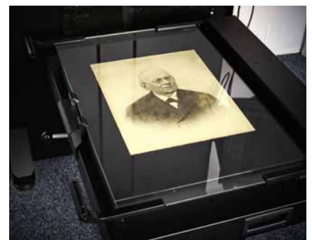
■ Photo table with glass plate and soft pad for very careful handling
