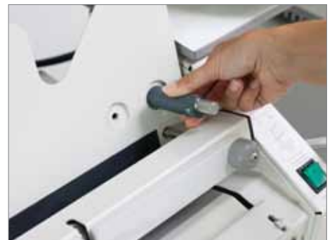
Predefined places for paper stopper. Optional hard cover guide set supports edge margins from 2.5 to 7.5 mm
